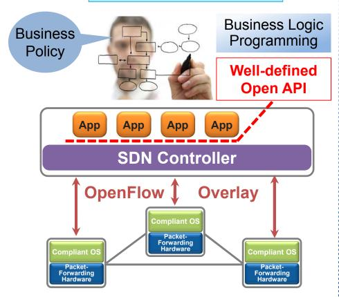
Separate control plane from the data plane in network devices (physical and virtual) with intelligence and programmability centralized in a controller.
